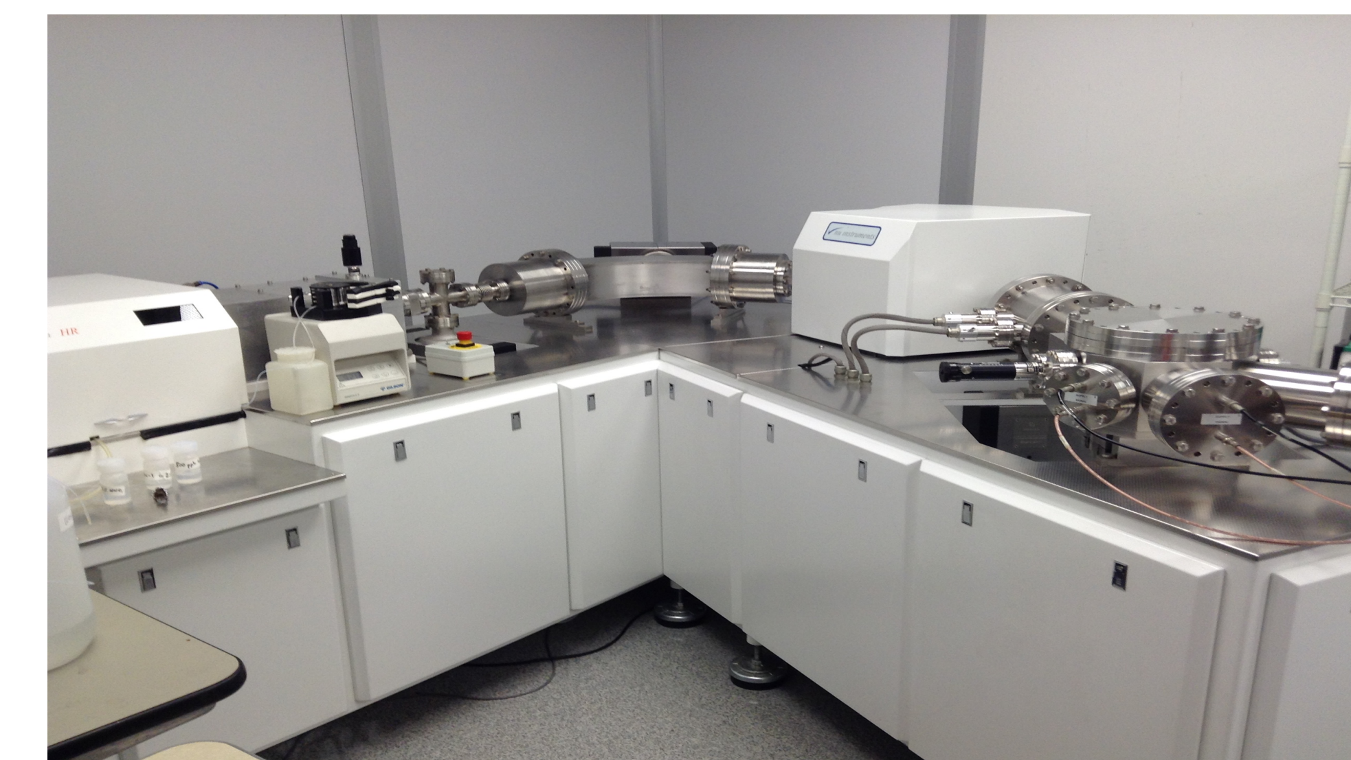
Figure 3. The Nu Plasma multi-collector inductively-coupled plasma mass spectrometer (MC-ICP-MS)
